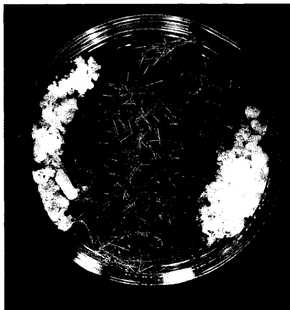
Fig. 1. Photograph showing the growth of the racemic compound of ephedrine, consisting of needles at the center of a glass petri dish, from vapors of the individual enantiomers kept diametrically separated. The crystals on the left are of l -ephedrine; those on the right are of d -ephedrine.
